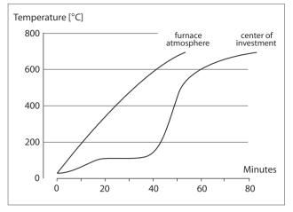
**Fig. 18-36 Thermal inertia** The investment accumulates energy during heating of the oven (i.e., heat soaking), hence the delay in temperature increase in the center of the investment. Data from Jelenko Corp.
